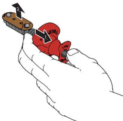
Fig. 131: Replacing the fusible link
