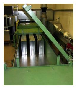
The test run, a double-walled, sound insulated and airtight stretch of channel, is attached to the reverberation chamber. The channel has a part where the channel width can be varied, which means that sound attenuator elements (splitters) of different widths and distances can be tested. Sound attenuator parameters such as insertion loss, air-regenerated noise and pressure loss are measured.
