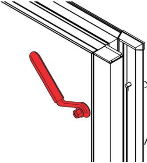
Fig. 5: Inside door handle on an inspection access door
