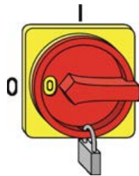
Fig. 8: Securing the mains isolator
