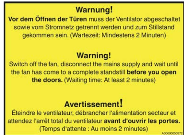
Fig. 1: Notice on inspection access doors
