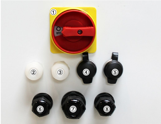
Fig. 32: Cable entry points below the mains isolator
